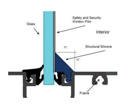
Improper Attachment System installation (curved bead):
