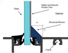
Internal testing indicates that a window with safety and security film with an attachment system provides improved protection against a would-be intruder compared to a window that has film applied without an attachment system.
